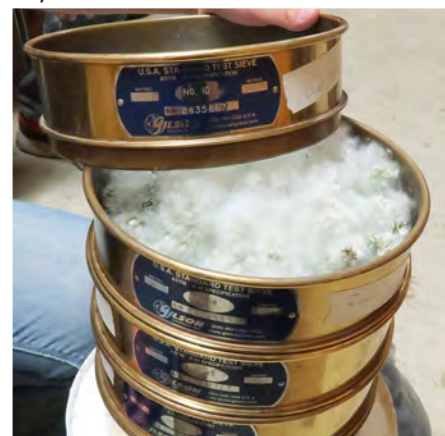
Photo 4: Place catkins and fluff in the second sieve. Blow air through the top sieve.
